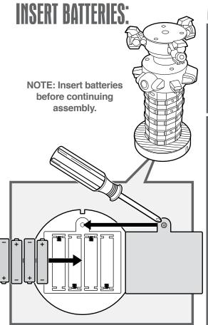
Using a Phillips/cross head screwdriver (not included), unscrew battery cover. Insert 4 fresh 1.5 V AA or LR6 size alkaline batteries. Replace battery cover and tighten screw.
